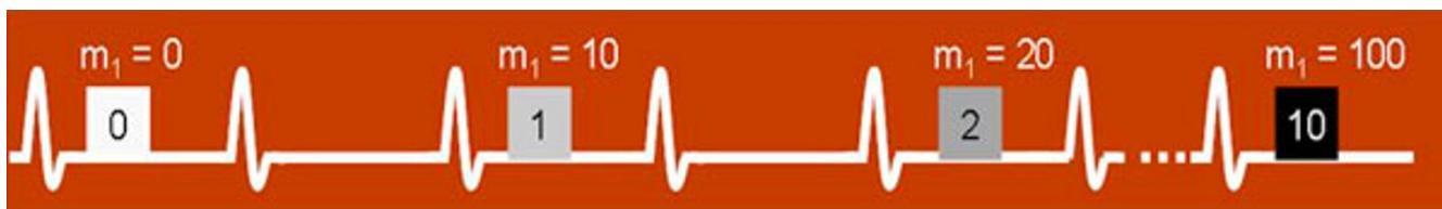
Figure 2 Schematic of the 2D m_1 -scout approach. A total of 11 images were collected within 1 min. The first uses m_1 = 0 , while the latter uses incremental m_1 values (user specified)
