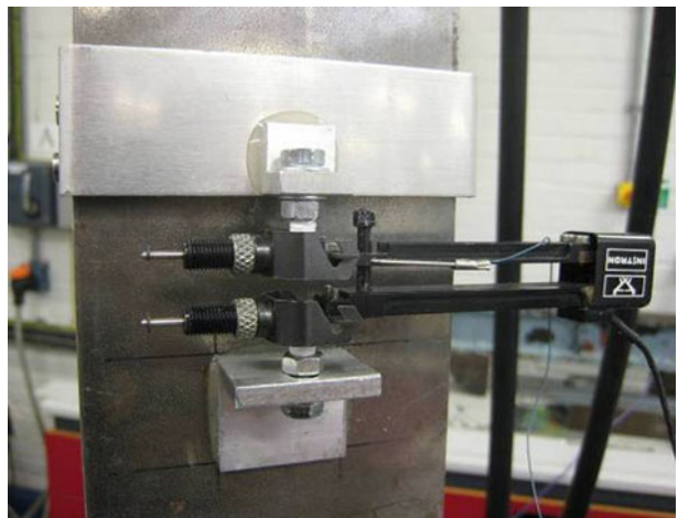
Fig. 2 Strain gage extensometer applied to bonding plates
