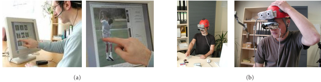
FIGURE 1: (a) Interactive content-based image retrieval using speech and haptics. (b) Head-mounted cameras and display for augmented reality visualisation of recognised objects and events in an office environment.
