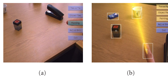
FIGURE 7: Office desk as seen through the mobile memory spectacles shown in Figure 1b. (a) Menu selection using pointing gestures. (b) Object referencing using pointing gestures.
