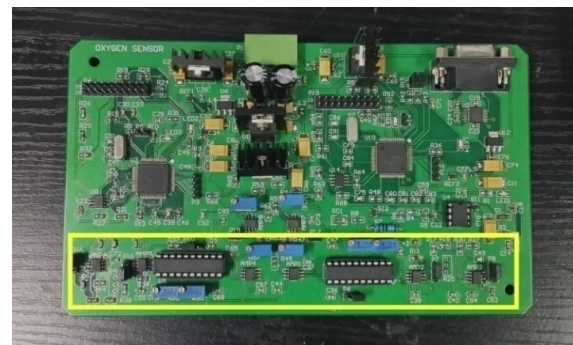
Fig. 4 Photo of fabricated oxygen detection system: the designed lock-in amplifier is under the picture, delimited by the solid line.
