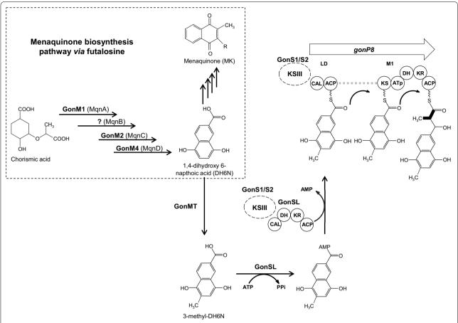
**Fig. 5** Proposed biosynthesis pathway of PM100117 and PM100118 naphthoquinone moiety. *LD* loading domain, *M1* extension module. Polyketide synthase domains are as follows *KS* ketosynthase, *AT* acyltransferase, *KR* ketoreductase, *DH* dehydratase, *ACP* acyl-carrier-protein, *CAL* CoA ligase, *KSIII* 3-oxoacyl-ACP synthase III
