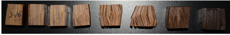
Fig. 5 Failure types of compressive strength parallel to grain at different temperatures. From left to right are the control sample and samples exposed to 50, 80, 110, 140, 170, 200, and 230 °C for 2 h
