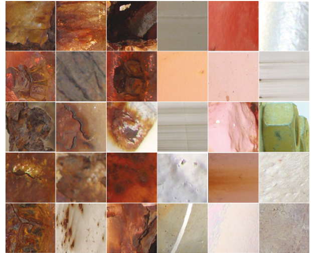
FIGURE 1: Image database. The three columns on the left illustrate metallic surfaces attacked by atmospheric corrosion. The three columns on the right illustrate a variety of smooth and rough non corroded surfaces.
