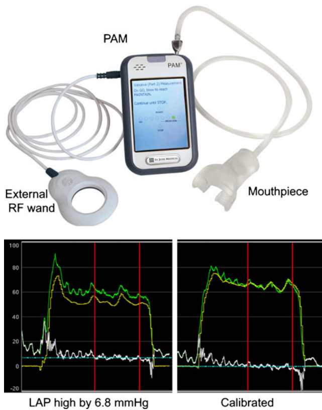
Fig. 2 Noninvasive calibration system and procedure. Top Patient advisor module (PAM) with atmospheric pressure reference transducer connected to the mouthpiece for airway pressure measurement during Valsalva maneuver. PAM display allows the patient to view effort during strain and subsequently displays Valsalva waveforms for acceptance. Bottom Valsalva waveforms uncalibrated and calibrated: LAP (green), airway pressure (yellow), differential pressure (white), measurement period (between red lines), offset drift (blue line)
