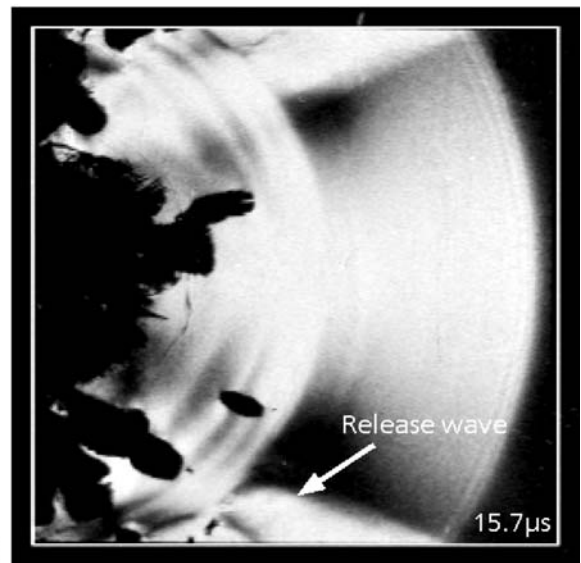
Fig. 8 A comparison of the longitudinal stress wave fronts obtained (a) computationally and (b) experimentally (in Ref 1, 2) for the case of a spherical impactor with an initial velocity of 440 m/s and a post-impact time of 15.7 \mu s
