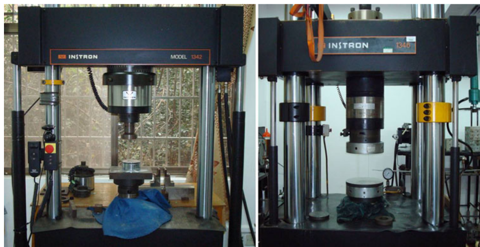
Fig. 3 The stiff test machines Instron 1342 and 1346 at Central South University
