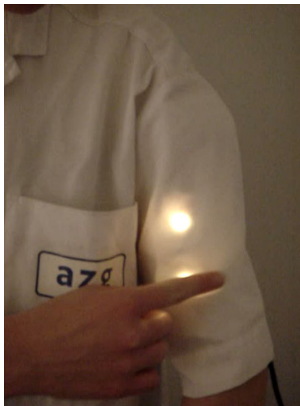
Fig. 3 Prototyped multisensory display as it was tested with nurses, under their clothes. It consisted of four RGB LEDs and vibrating elements. It was coded in MAX/MSP and signalled a rhythmic pattern accompanied by one of three different colours. It has a push button to stop and a sound element (for private sounds). The elements were placed in soft cloth under the clothes
