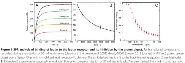
B) Example of a sensorgram recorded during buffer flow after complete injection of 30 nM leptin (black). The pink dashed line is a fit to the data using equation 1 (see Methods). The two vertical lines occur during the extended time dissociation when the machine switches between its two pumps.
