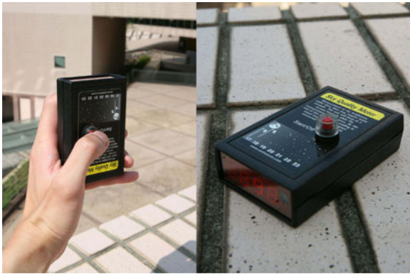
Fig. 2 The Sky Quality Meter: the light sensor is located on the side of the near-infrared filter next to the display
