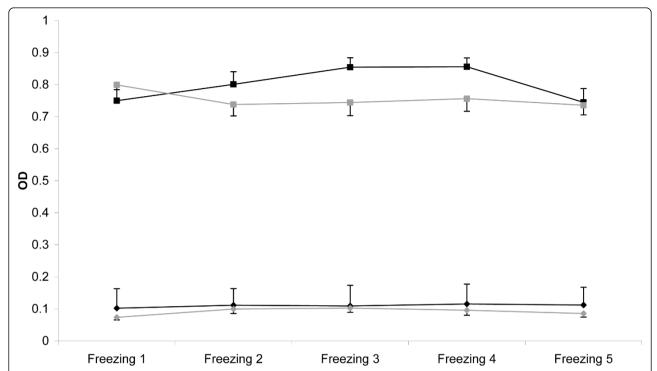
**Figure 1 Optical densities (OD) through five freeze-thaw cycles**. Mean optical densities (OD) for positive (black diamonds) and negative (black squares) clean sera, and for positive (grey diamonds) and negative (grey squares) haemolysed sera (± standard error, SE) through the five freeze-thaw cycles (Freezing 1 to 5).
