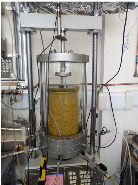
Fig. 1 Photo of one-third scale ballast specimen of height = 300 mm and diameter = 150 mm in a GDS Instruments [10] triaxial apparatus. The triaxial cell was mounted within a reaction frame and bolted to a pedestal seated by self-weight onto a bottom-up mechanical drive unit used to apply axial strain or stress
