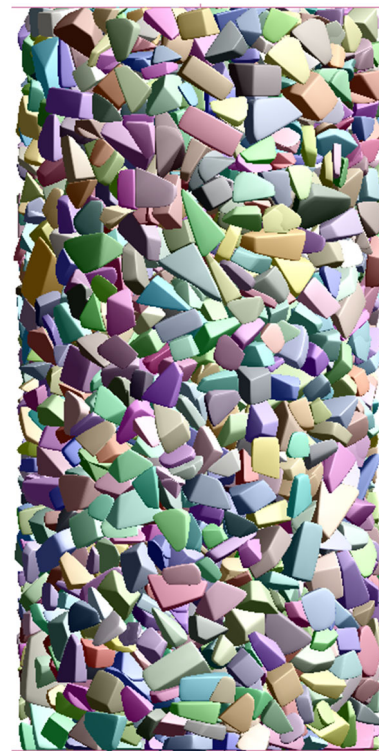
Fig. 4 Image of numerical triaxial specimen, showing potential particle representation of railway ballast
