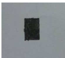
Fig. 4 ESL49000 material as the sacrifice layer.
