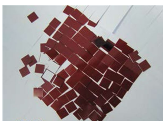
Fig. 2 Polyimide material as the sacrifice layer.
