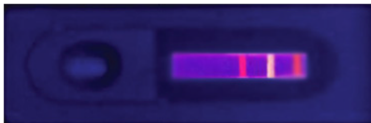
Fig. 4 Direct observation of the strip added with 20 ng/mL PCT and 2 \mu\text{g/mL} CRP
