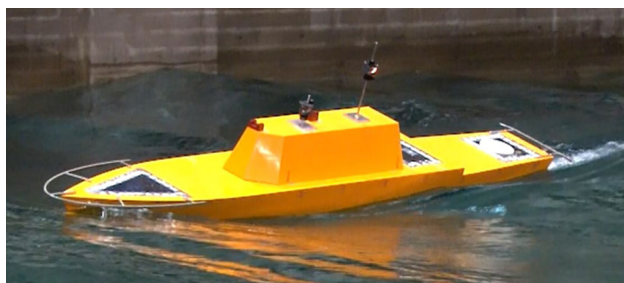
Fig. 5 Photograph of the ship model of ONR flare topside vessel during the experiment
