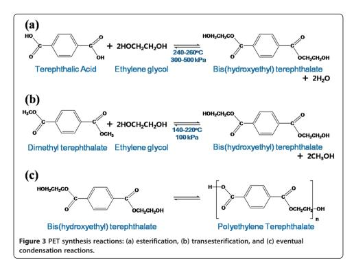
1960s. The PET, up to this stage, is appropriate for applications such as fibers and recording tapes for which high molecular weight or viscosity is not required. PET with high molecular weight and viscosity for bottles or technical yarns is produced by further polycondensation through the solid-state polymerization process.
