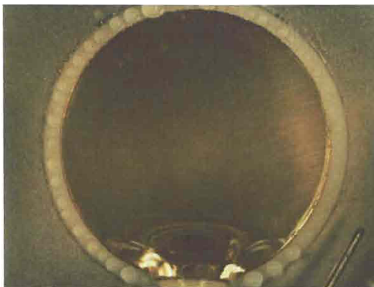
Fig. 7 Filmwise condensation of steam on a 2 000 nm thick electrodeposit of the 65 gold/25 copper/10 cadmium weight per cent alloy from an alkaline cyanide bath
