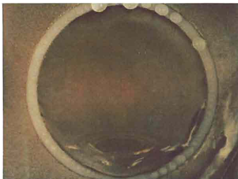
Fig. 6 Perfect filmwise condensation of steam on solid, pure gold which had been heated to 593°C for 1 hour and quenched
