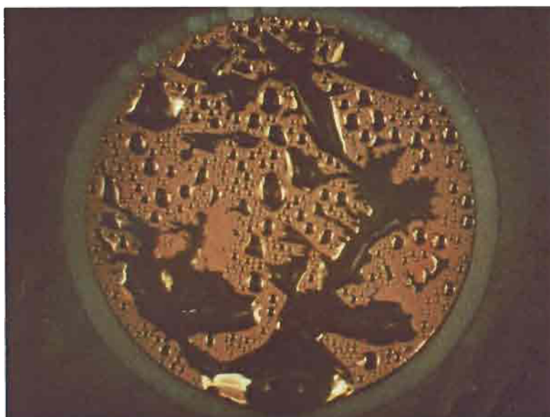
Fig. 5 Mixed condensation of steam on a 100 nm thick gold electrodeposit from a cyanide bath without brightener
