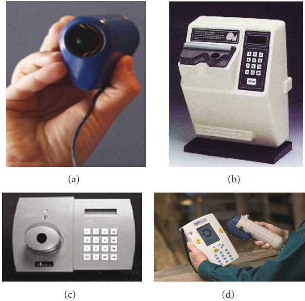
FIGURE 3: Some retinal scanners, (a) a human retinal scanner, (b) and (c) human retinal recognition scanners, and (d) a cow retinal scanner.
