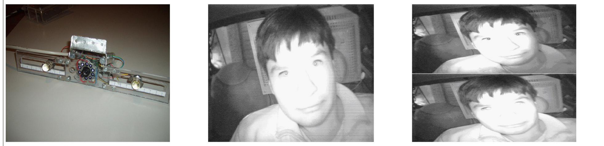
Figure 27 Perception system using infrared illumination (a) vision system, (b) drivers image, and (c) odd (top) and even (bottom) image fields.
