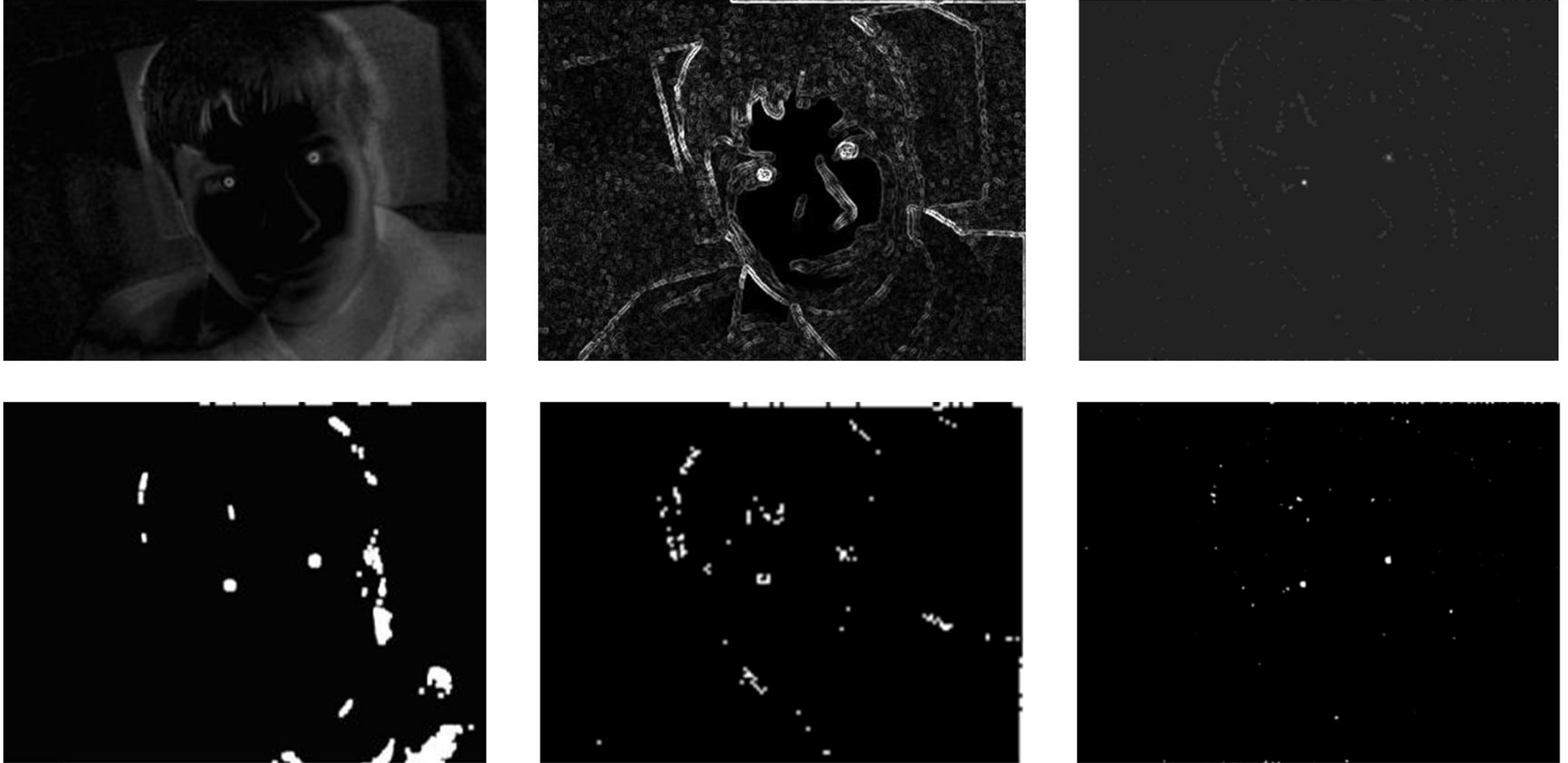
Figure 28 Difference (a), edge (b), and FRST (c) and their binary images (d), (e) and (f), respectively.
