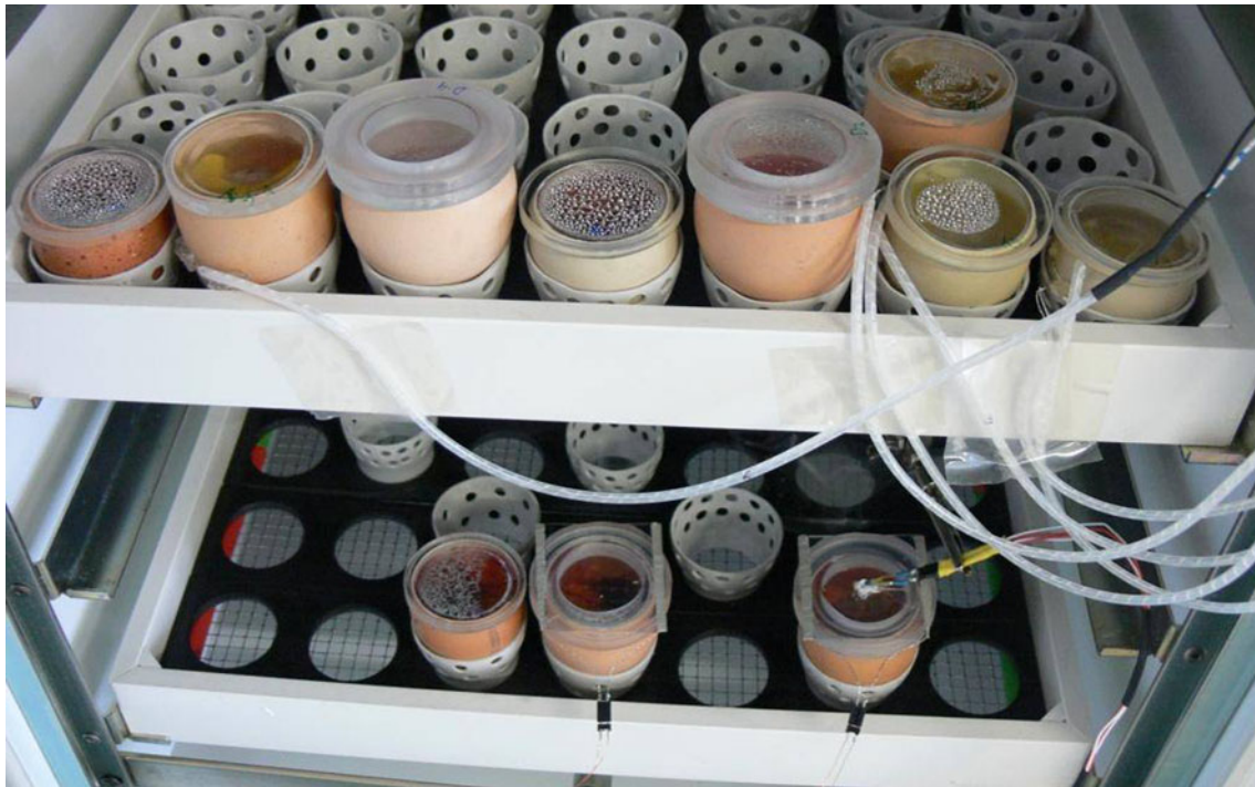
Fig. 5 Experimental setup for thermal measurement of developing chicken embryo with thermocouple. Measurement of allantoic fluid temperature as an index of deep body temperature of developing
