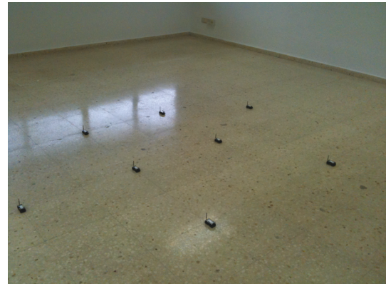
FIGURE 4: Arrangement of nodes in the localization test.
