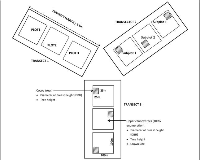
**Fig. 2** Layout of transects, main plots (100 m  $\times$  100 m) and subplots (25 m  $\times$  25 m) in each study district. *Lower arm* of *Y*-shape (Transect 3) shows dimensions of main and subplots and parameters measured (for both cocoa and shade trees) within each transect. Each transect is 5 km long and minimum distance between plots is 500 m
