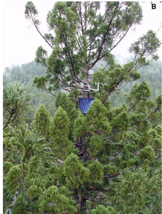
Fig. 5 Using newly developed, safe, and reliable canopy access techniques, we can make the same measurements in the canopy as we do on the ground. a Measuring the trunk diameter of a Cryptomeria japonica tree at 15 m above ground in Yakushima Island, Japan (Photo: H. I.). b Micrometeorological sensors installed atop a 111-m Sequoia sempervirens tree in California (Photo: S.C. Sillett)
