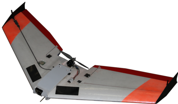
Fig. 1. Picture of NPS ZephyrII UAV, a low-cost yet capable system leveraging open-source and commercially available components.
