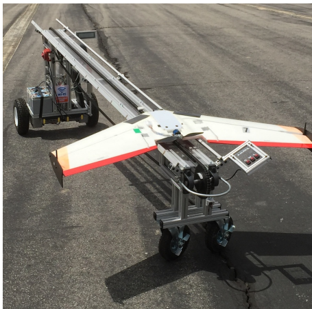
Fig. 5. Picture of the ARSENAL Automated Multi-Plane Propulsion System (AMPPS) robotic launcher, used in the 50-UAV mission for rapid launch. AMPPS uses an electric motor to launch the UAV, and is equipped with, e.g., ROS-enabled sensors, differential drive motors, and gamepad for triggering launch and teleoperation.
