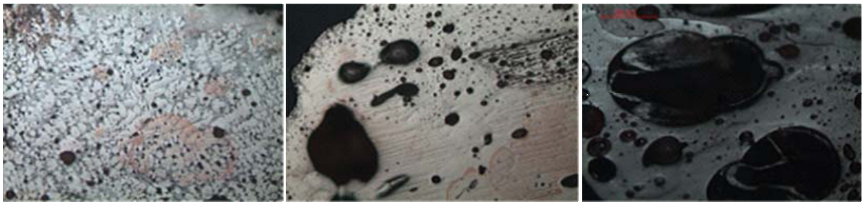
Fig.4-2 Three short circuit conditions melted bead (300A 100X)
