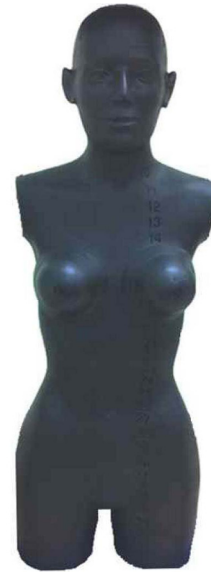
Fig. 2. Frontal View of the RANDO ® Female Phantom.
