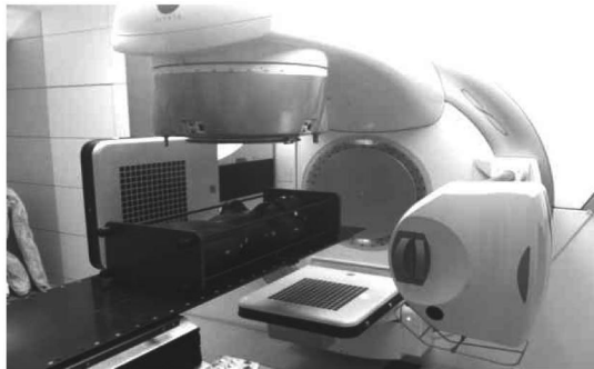
Fig. 1. Elekta Infinity System Equipped with XVI CBCT System and RANDO Physical Phantom Placed on the Patient Bed
