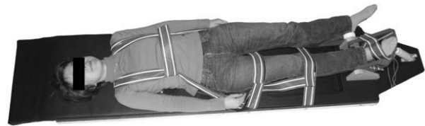
Fig 1. The self-built exercise bench permits isotonic stress exercises of the calf muscle with a defined workload, which is measured via force at the piston and via distance and is adjusted by a feedback control system. The volunteer lying on the exercise bench indicates the correct positioning for the phosphor 31 magnetic resonance spectroscopy examination.
