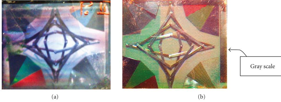
FIGURE 7: Reconstructed images of a test object from a single layer (a) and two layers (b) reflection holograms recorded on ultrafine grain light sensitive material HP-P.
