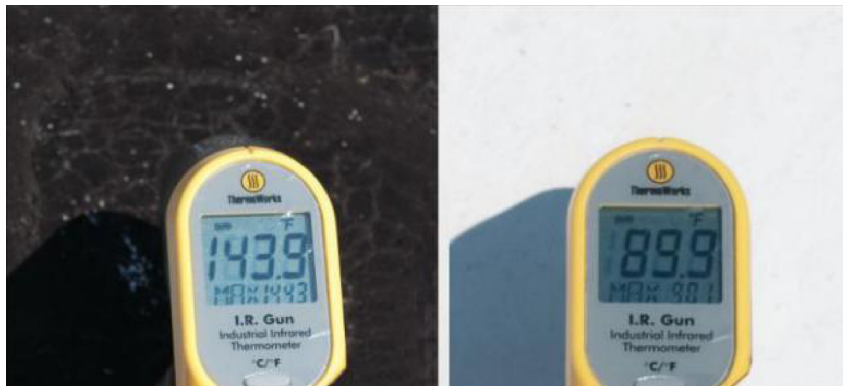
Figure 8 Dark vs. cool roof surface. temperatures. (Urban and Roth, 2010).
