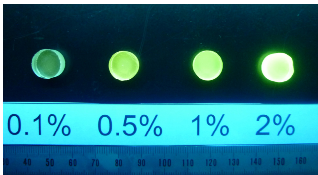
Fig. 11. Green PL emission from \text{Tb}^{3+} ions in Tb–P codoped samples (Tb to Si molar ratios ranging from 0.001 to 0.02 at a P to Tb molar ratio of 1) exposed to UV light (254 nm) from a mercury lamp.
