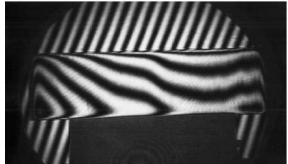
Fig. 9. Photograph of a He–Ne interference pattern through a Nd–Al codoped silica glass ( \text{Nd}_2\text{O}_3 , 1.25 wt.%; \text{Al}_2\text{O}_3 , 2.72 wt.%), sized 93 \text{ mm} \times 28 \text{ mm} \times 11 \text{ mm} , prepared by sintering aluminosilicate zeolite powders loaded with \text{Nd}^{3+} ions. The optical quality is sufficiently good for the amplification experiment.
