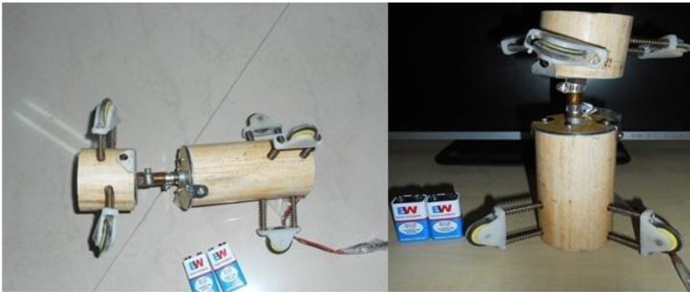
Fig.8. Rough prototype of new in-pipe inspection robot
