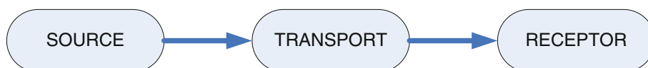
Fig. 1 The concept of risk/impact illustrated as a chain of events. For a risk or impact to occur, the chain must remain unbroken, and an undesired effect must occur at the receptor
