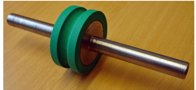
Fig. 8. High-friction feeding wheel used in the constructed cable feeder prototype.
