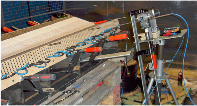
Fig. 12. Experimental setup used for validating the cable feeder tool function with a full scale UU WEC stator section.
