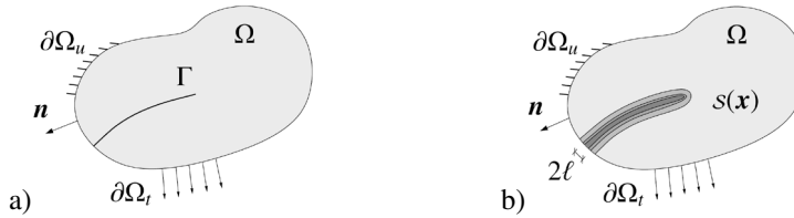
Fig. 1. Elastic body with (a) a sharp crack \Gamma \subset \mathbb{R}^{ndm-1} and (b) a phase field approximation s(x) of the crack by a smooth transition between s = 1 for intact material far away from the crack and s = 0 for the fully broken state of material in the crack.
