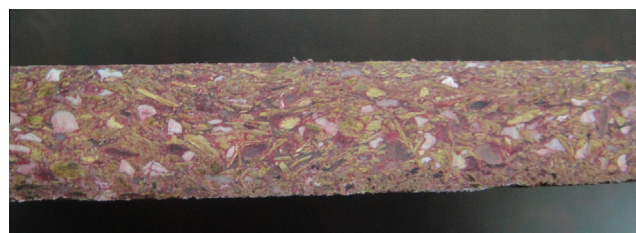
Fig. 3. Cross-section view of wood plastic.
