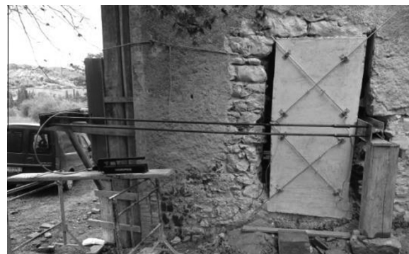
Fig. 2. On-site shear-compression test (Colle Umberto building).
