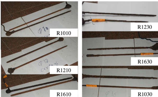
Fig. 5 The external surface of corroded bare bars.
