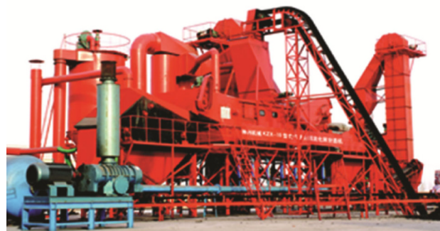
Fig. 2 Modularized industrial-scale ADMFB separator
