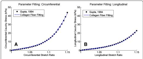
**Figure 4 Fitting of material properties to experimental data.** The properties of the scar tissue were fit to experimental data obtained by Gupta, et al. 1994 for a 6-week old porcine infarct. **(A)** The fitting to the circumferential stress resulted in an  $R^2$  value of 0.996. **(B)** The fitting to the longitudinal stress resulted in an  $R^2$  value of 0.994.
