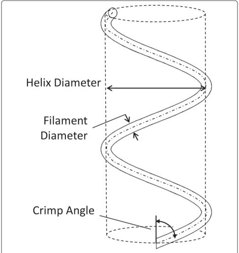
**Figure 2 Schematic of crimped collagen fiber.** The collagen filament coils around a central axis that is aligned in the fiber direction. The diameter of the filament, the diameter of the fiber helix, and the crimp angle are illustrated.
