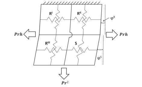
**Figure 3 Schematic of force division and balance.** The LV is modeled as a system of springs with a longitudinal and circumferential spring for each of the four regions. Springs shown in parallel share displacements and springs shown in series share forces. The applied forces are calculated from the Law of Laplace.
