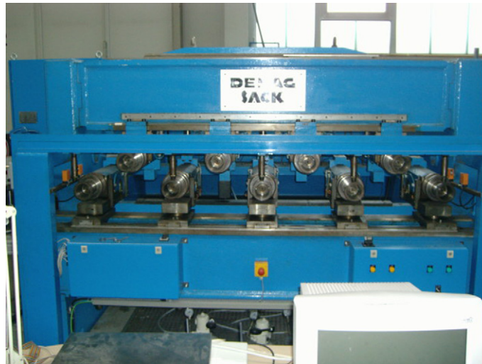
Fig. 3. Straightener pilot plant used to validate the methodology (photo courtesy of Betriebsforschungsinstitut, BFI).
