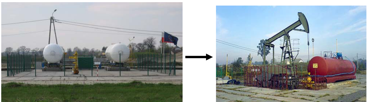
Figure 2 Picture showing the conversion of MS-3 well from injector (left) to producer (right)
