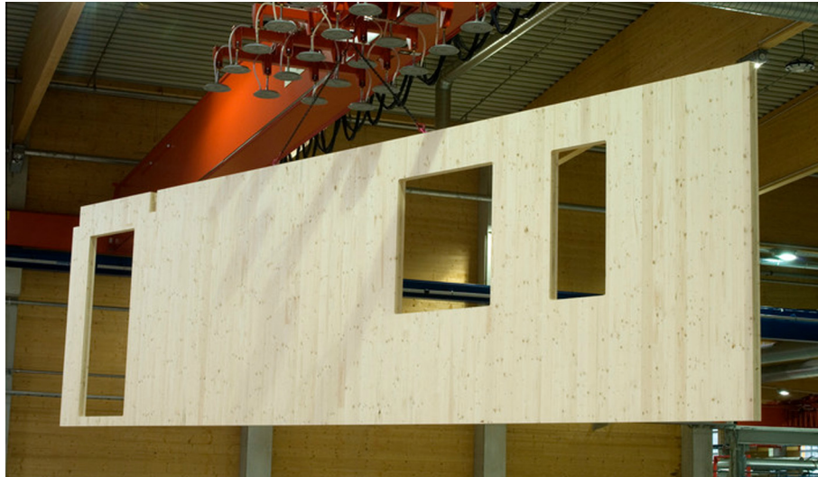
Fig. 1. CLT panel under construction. Source: Stora Enso.
