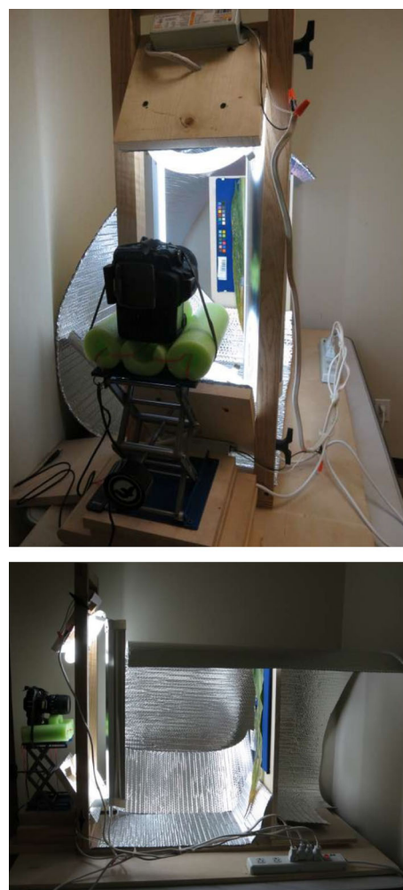
Fig. 3 Jig used for image capture. Views from front ( top ) and side ( bottom )
