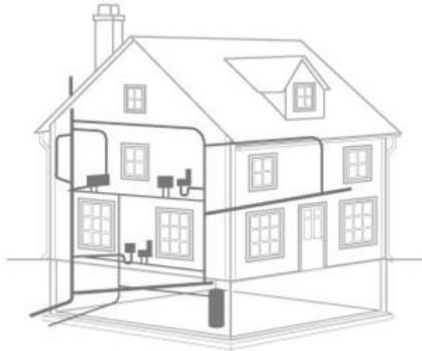
Fig. 2: Basic piping layout in a normal household
