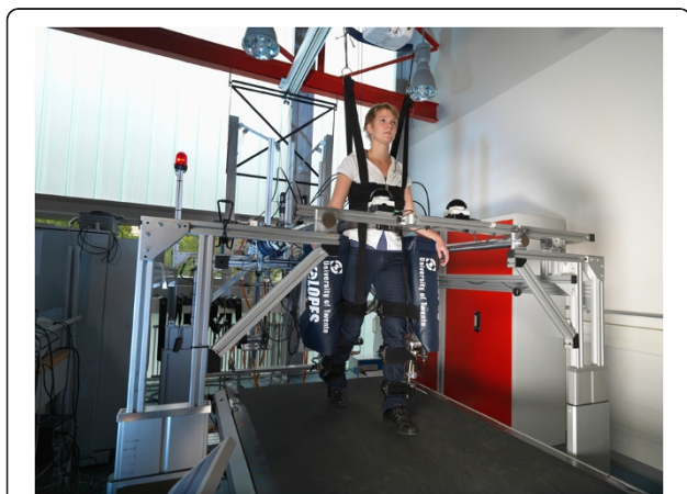
Figure 3 The prototype of the gait rehabilitation robot LOPES.
