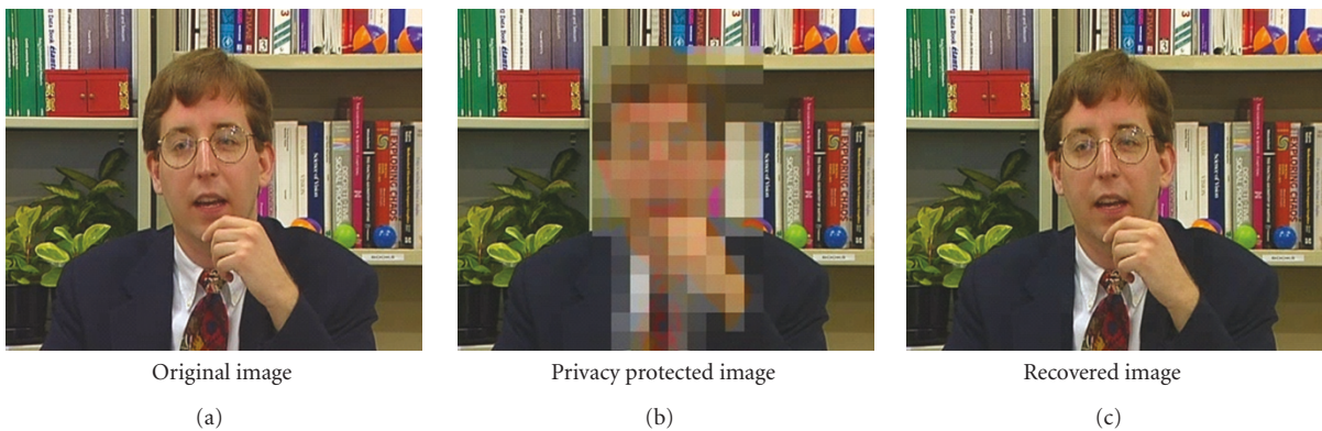
FIGURE 7: Video sequence: deadline ( 352 \times 288 ), DWT level: j = 4 , quantization step size: \Delta = 1 , compression: JPEG.
