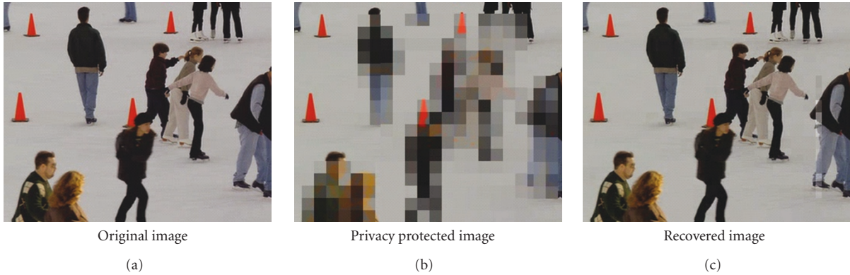
FIGURE 6: Video sequence: ice ( 352 \times 288 ), DWT level: j = 4 , quantization step size: \Delta = 1 , compression: JPEG.
