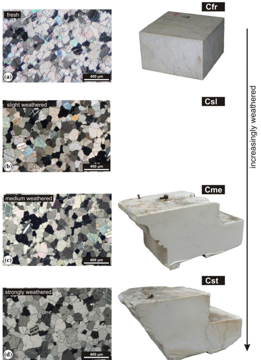
Fig. 4 Investigated samples of Carrara marble: weathered specimens from the Marble Palace in Potsdam and a fresh reference sample from the quarry near Gioia (Italy)
